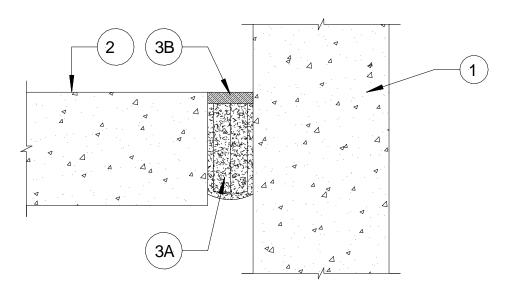
1. **Wall Assembly** – Min 8 in. (203 mm) thick reinforced lightweight or normal weight (100 – 150 pcf or 1600-2400 kg/m³) structural concrete. Wall may also be constructed of any UL **Classified Concrete Blocks**\*.
