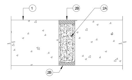
1. **Wall Assembly** – Min 5-3/4 in. (146 mm) thick reinforced lightweight or normal weight (100 – 150 pcf or 1600-2400 kg/m³) structural concrete. Wall may also be constructed of any UL Classified **Concrete Blocks**\*.
